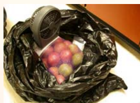
Figure 1. Design of mesh bag inside of poly drum liner tests. For testing, the liner is pulled up and filled with air from a standard lab source, then sealed for treatment.
