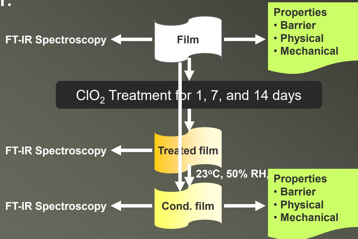
**Scheme 2.** Flow Diagram of Chlorine Dioxide Treatment of Packaging Materials
