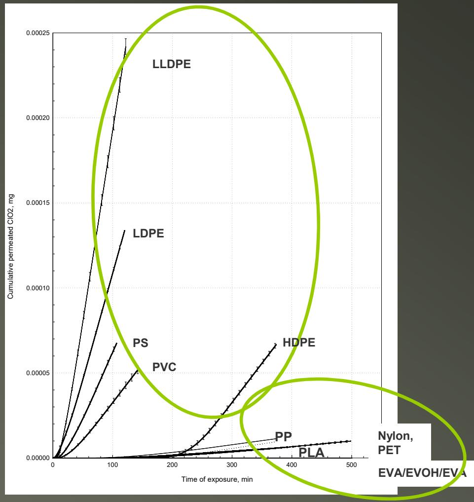
**Figure 2.** Mass transfer of 10 mg  $\text{ClO}_2/\text{L}$   $\text{ClO}_2$  gas through polymeric packaging material
