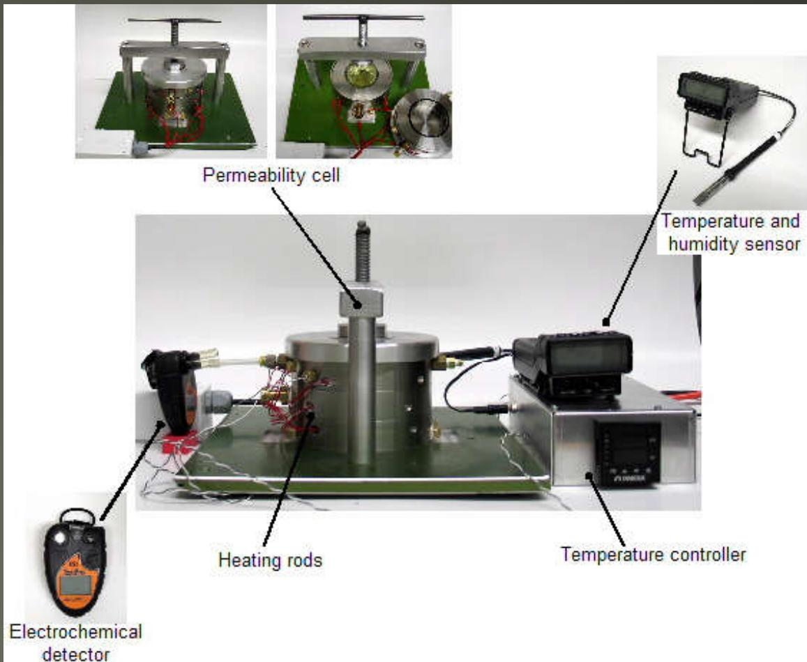
**Figure 1.** Setup of Continuous System for Measuring  $\text{ClO}_2$  mass transfer
