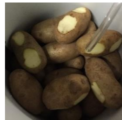
Figure 1.2 Wounded potatoes- wounded potatoes were located in three layers: bottom, middle and top. (4 potatoes per layer). They were randomly placed in each layer.
