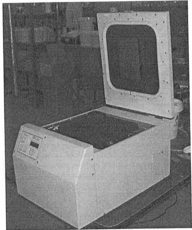
Figure 2. ClO 2 Clave unit designed for ClO 2 gas treatment studies
